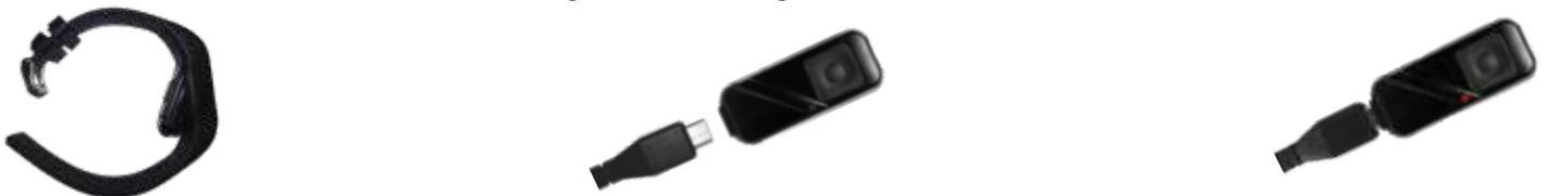
While charging, the red LED will be steady on, once the charge is completed the LED will become green. At this point it will be possible to wear SMAIRTHERO. It is possible to use any USB type charger, which has indicated in the "5V output" specifications and that can supply a minimum current of 2.0 A. Check that the USB power adapter is approved for safety (indicated by "LPS", "Limited Power Supply", "UL listed" or "CE").
