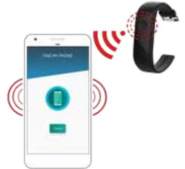
To activate the phone search it is sufficient that SMAIRTHERO is connected to the smartphone; in fact it is not necessary that the SmairtHero service is active.
