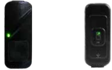
At the top of it there is a button and a multicolor LED, and inside of it there is a buzzer (acoustic signaller).
